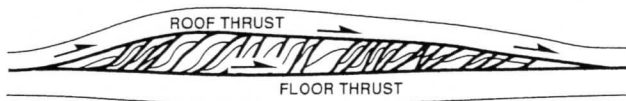
Figure 31. Smooth roof duplex where the roof thrust varies smoothly without folding by the underlying link thrusts (adapted after McClay & Insley 1986).
