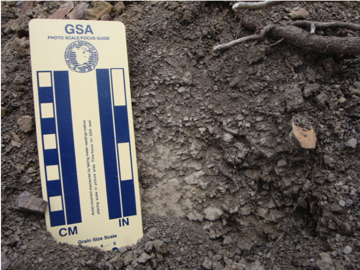
Figure 15. Inferred fault gouge found at Saruche Canyon lineament.
