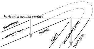
cross section through a fold with an overturned limb
