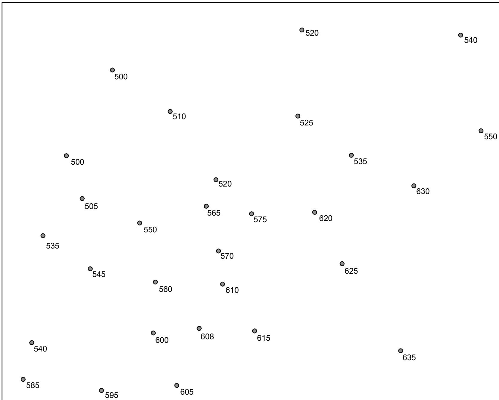
Contour the elevation data at an interval of 10 and infer the location of any faults in the map area.
