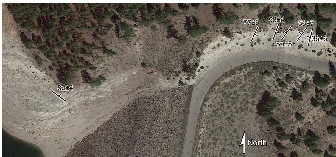
Figure 16. Aerial map view of the faults present in the northeast abutment of the Stampede Dam. The strike-and-dip symbols on the upper right corner of the image are faults 1-5, as labeled in figure 14 above. Orientation data for fault 8 is shown on the left (west) side of the image, and faults 9-11 are in that same area. The road in the image is Dog Valley Road. Image was taken 16 April 2015 and was acquired from Google Earth.
