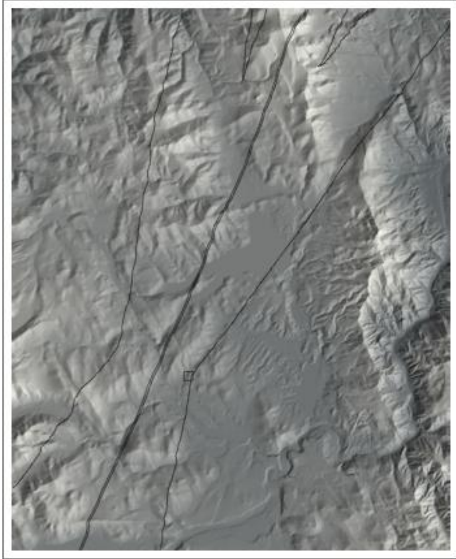
Figure A5. Raw output of SLAMcode.nb for earthquake A4 on 6 August 1993. Small square marks the epicenter at latitude 39.41621^{\circ}\text{N} longitude 120.18018^{\circ}\text{W} . Nodal plane dip direction is 115^{\circ} , dip angle 50^{\circ} , rake -70^{\circ} . Hypocenter depth was 0.368 km. The curves indicate the extent of the seismo-lineament. The image is aligned with the UTM grid, so the image would have to be rotated \sim 1.73^{\circ} clockwise to be aligned with the geographic coordinate system at/near its center. North is toward the top of the page.
