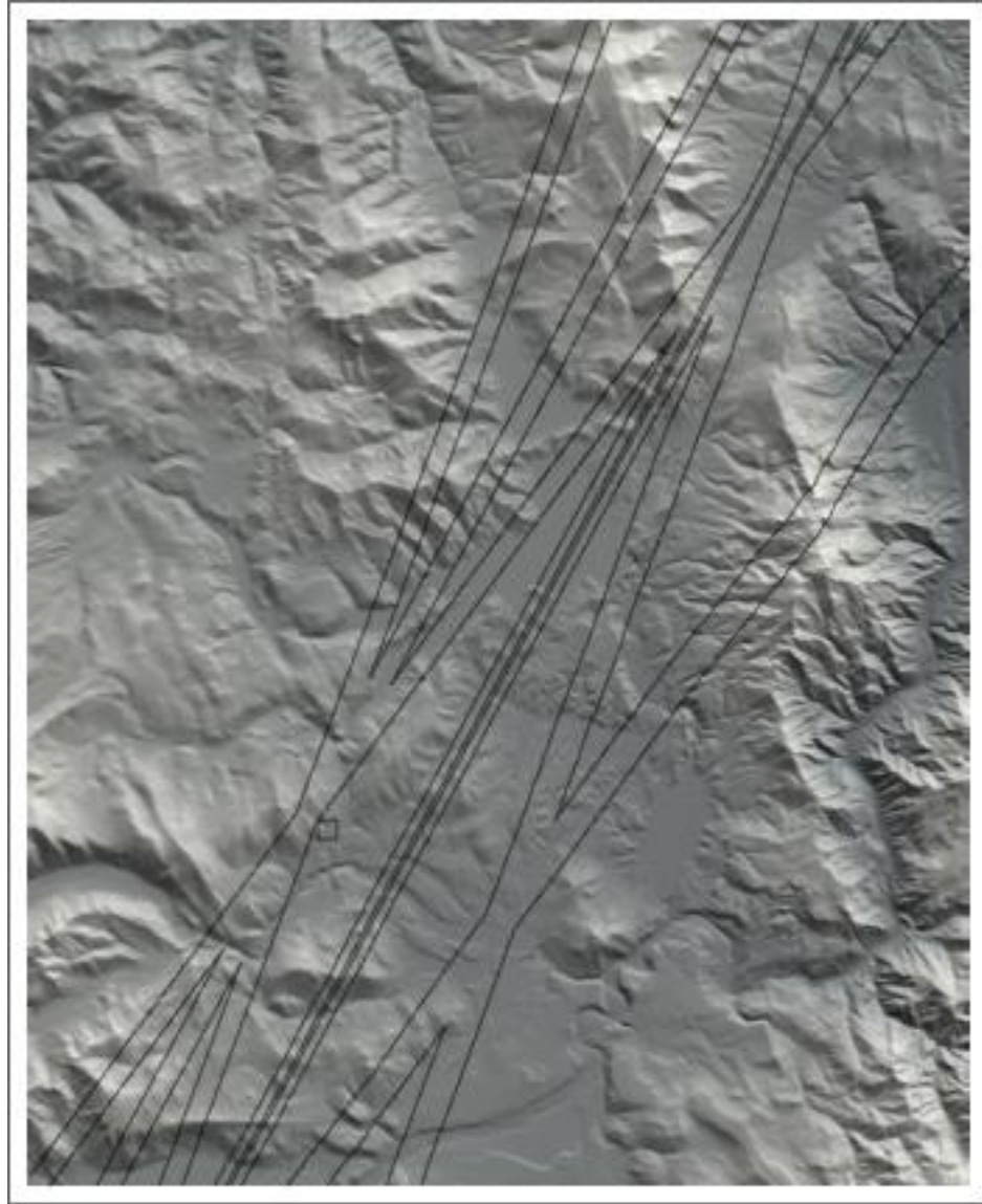
Figure A2. Raw output of SLAMcode.nb for earthquake A2 on 3 July 1983. Small square marks the epicenter at latitude 39.412^{\circ}\text{N} longitude 120.206^{\circ}\text{W} . Nodal plane dip direction is 300^{\circ} , dip angle 80^{\circ} , rake 20^{\circ} . Hypocenter depth was 11.05 km. The curves indicate the extent of the seismo-lineament. The image is aligned with the UTM grid, so the image would have to be rotated \sim 1.73^{\circ} clockwise to be aligned with the geographic coordinate system at/near its center. North is toward the top of the page.
