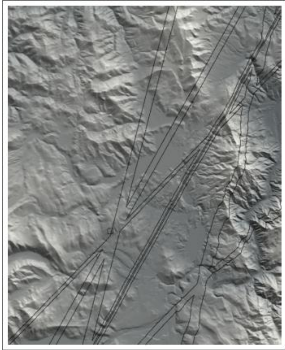
Figure A3. Raw output of SLAMcode.nb for earthquake A3 on 30 August 1992. Small square marks the epicenter at latitude 39.42047^{\circ}\text{N} longitude 120.18852^{\circ}\text{W} . Nodal plane dip direction is 301^{\circ} , dip angle 61^{\circ} , rake 12^{\circ} . Hypocenter depth was 5.34 km. The curves indicate the extent of the seismo-lineament. The image is aligned with the UTM grid, so the image would have to be rotated \sim 1.73^{\circ} clockwise to be aligned with the geographic coordinate system at/near its center. North is toward the top of the page.
