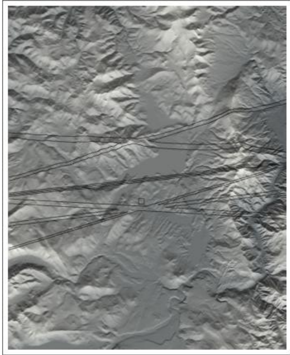
Figure A9. Raw output of SLAMcode.nb for earthquake A5 on 15 January 1998. Small square marks the epicenter at latitude 39.44810^{\circ}\text{N} longitude 120.15511^{\circ}\text{W} . Nodal plane dip direction is 175^{\circ} , dip angle 73^{\circ} , rake 121^{\circ} . Hypocenter depth was 4.636 km. The curves indicate the extent of the seismo-lineament. The image is aligned with the UTM grid, so the image would have to be rotated \sim 1.73^{\circ} clockwise to be aligned with the geographic coordinate system at/near its center. North is toward the top of the page.
