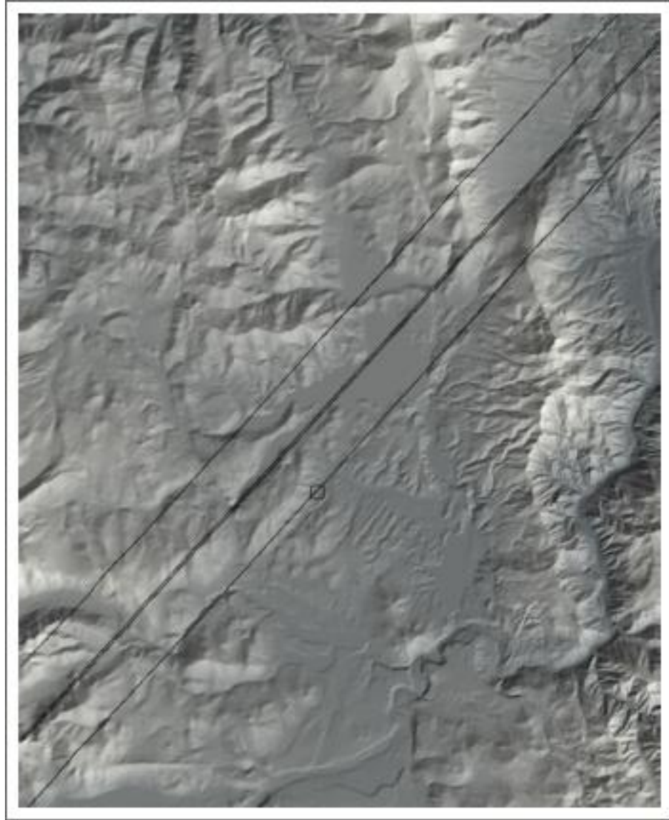
Figure A1. Raw output of SLAMcode.nb for earthquake A1 on 12 September 1966. Small square marks the epicenter at latitude 39.438^{\circ}\text{N} longitude 120.160^{\circ}\text{W} . Nodal plane dip direction is 134^{\circ} , dip angle 80^{\circ} , rake 180^{\circ} . Hypocenter depth was 10 km. The curves indicate the extent of the seismo-lineament. The image is aligned with the UTM grid, so the image would have to be rotated \sim 1.73^{\circ} clockwise to be aligned with the geographic coordinate system at/near its center. North is toward the top of the page.
