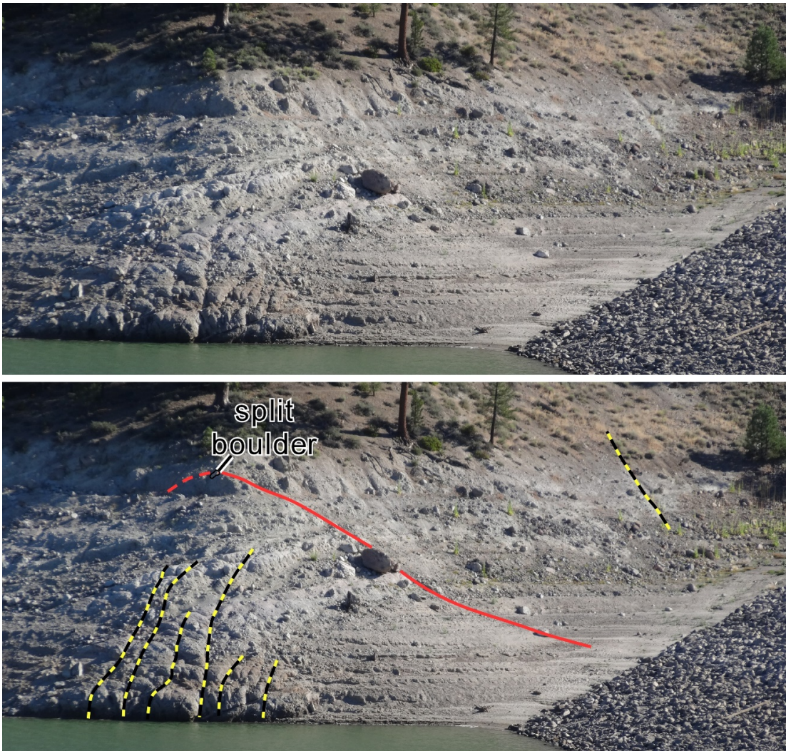
Figure 20. Photograph of fault 8 and related fractures taken from the Stampede Valley Dam looking north. Red curve is fault 8, yellow-black dashed curves are other joints or small faults. The location of the small split boulder used to obtain fault orientation data is shown.
