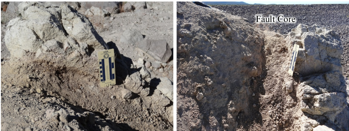
Figure 21. Photograph of the excavated fault core of fault 8. Fault core is ~15cm wide. Fault orientation data were obtained from both the excavated surface of the fault (left of center) and the face of a small split boulder (right of center).
